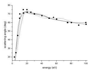
Fig. 2. Position of low-angle differential cross-section minimum versus incident energy for elastic electron scattering from argon. Experiment:  $\blacktriangle$ , Kessler et al. (1976); •, Srivastava et al. (1981);  $\Box$ , Panajotović et al. (1997). Theory: —, present results; …, Nahar and Wadhera (1987); - - -, Fon et al. (1983); · - - - , McEachran and Stauffer (1983).
