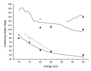
Fig. 5. Positions of differential cross-section minima in elastic electron scattering from zinc. Theory: —, present; - - -, McGarrah et al. (1991). Experiment: •, Predojević et al. (2000); ×, Williams and Bozinis (1975); +, Childs and Massey (1933).
