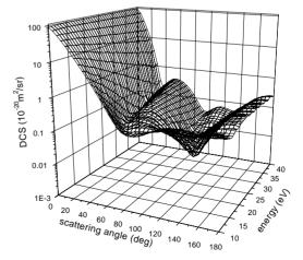
Fig. 4. Three-dimensional plot of the differential cross-section for elastic electron scattering from zinc.
